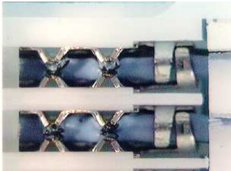
FIG.11 - IDC connector 3.5 mm pitch terminated onto 0.50mm 2 wires
