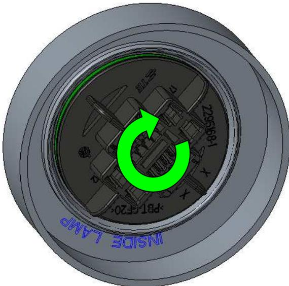
TURN THE CONNECTOR CLOCKWISE UNTIL STOP WHILE KEEPING PUSHING
