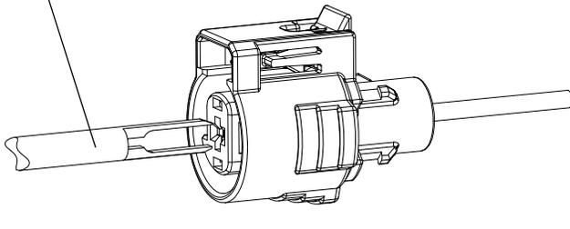
Pull Rearward on Wire While Tool is Inserted
