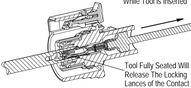
Tool Fully Seated Will Release The Locking Lances of the Contact
