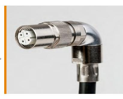
TE Connectivity (TE) introduces the M12 Rail 90° cable connector, a field installable connector developed for fault-free data transfers in harsh environments. This connector is specifically suited for harsh conditions due to the crimp termination of the signal contact and cable shield. The 90° design accommodates applications with limited available space for the cable exit.
