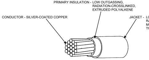
JACKET - LOW OUTGASSING, RADIATION-CROSSLINKED, MODIFIED PVDF Thickness: .003 ± .001 in.
