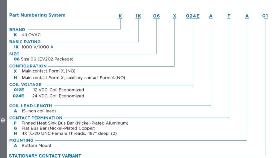
(2) User furnished bus bar must be equivalent to 4X 4/0 conductor. Torque to 45-55 in-lbs. per connection (5.1 - 6.2 NM)
