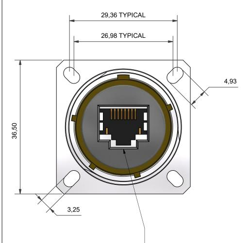
45,00 21,50 1.250-0.1P-0.3L-TS Ø28,00 LASER PART/BATCH MARK HERE
