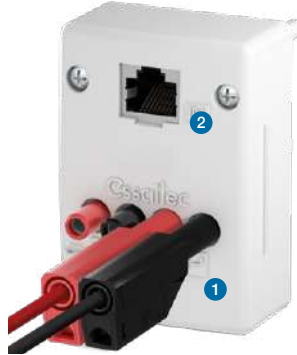
3.2 The ESSAILEC® RJ45 test plug has built-in dia. 4 (1) and RJ45 test sockets (2) in order to simplify the test operations. They allow current and voltage sensors measurement (1) as well as injection to the protection relay (2) .
