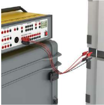
3.1 The test equipment is equipped with dia. 4 test plugs .
