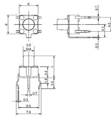
Dimensions are in millimetres unless otherwise specified.
