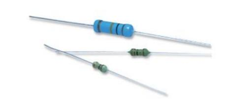
The resistive element comprises a thin film of nickel-chrome alloy evaporated onto a high thermal conductivity ceramic element. Metal end caps are force fitted to the element prior to spiralling to value. Tinned copper lead wires are welded to the end caps and the components are then coated. One coat of phenolic resin is followed by three coats of epoxy resin. All resistors are tested for value and tolerance.
