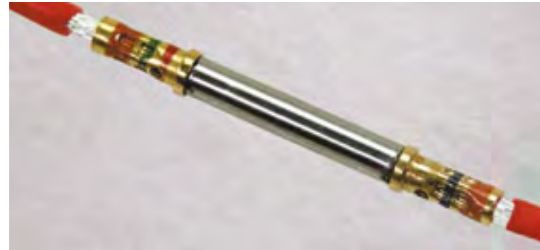
An example of a good crimp showing the exposed wire
