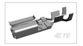
Terminal Type: Receptacle Mating Tab Width: 5.16 mm [.2 in ] Mating Tab Thickness: .85 mm [.034 in ] Terminal Transmits: 0 – 24 A (Low Power) Wire Size: 19 – 14 AWG
