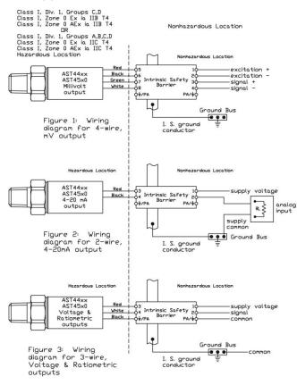
The transducers listed below are designed for installation in EITHER Class I, Division 1, Groups C,D; Class I, Zone 0 Group IIB DR Class I, Division 1, Groups A,B,C,D; Class I, Zone 0 Group IIC hazardous locations when connected to Associated Apparatus as described in note 1.
