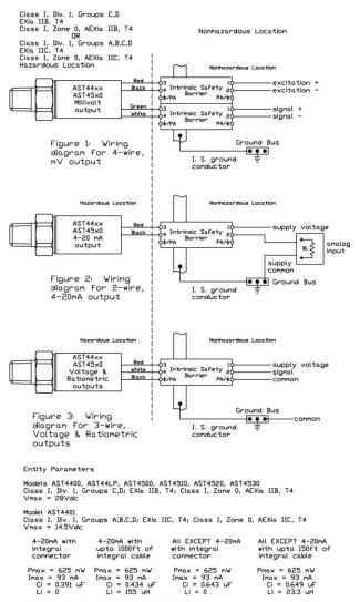
For installation in accordance with Fig 2, barrier must be a CSA Certified, Single Channel grounded Shunt-Blode Zener Barrier or a Single Channel Isolating Barrier.
