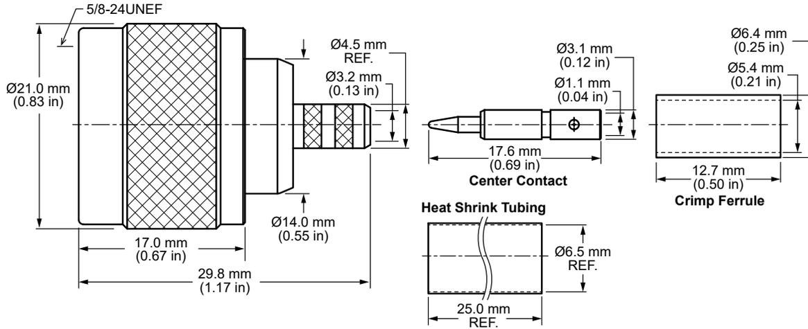
Figure 1: Product Dimensions for the CONN007-3-W Connector
