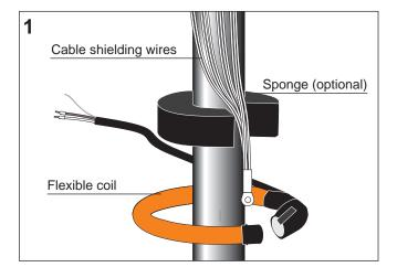
Close the flexible coil using its latching system.
