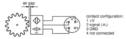
mates with straight plug M12x1, 4 pins
