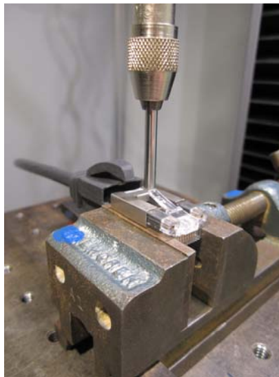
Figure 8 – Plug Latch Deflection Force Test Setup
