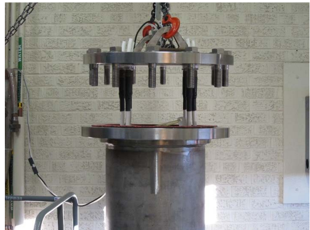
Figure 22 – Cable Assemblies Being Lowered Into Pressure Vessel
