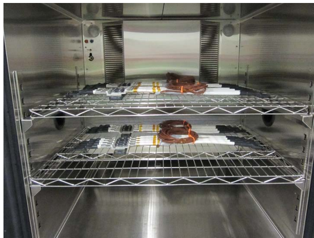
Figure 8: Cable Assemblies Loaded Into Humidity/Temperature Cycling Chamber
