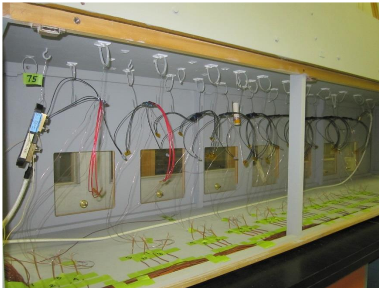
Figure 4 - Typical Temperature at Specified Current test setup (wire to wire).
