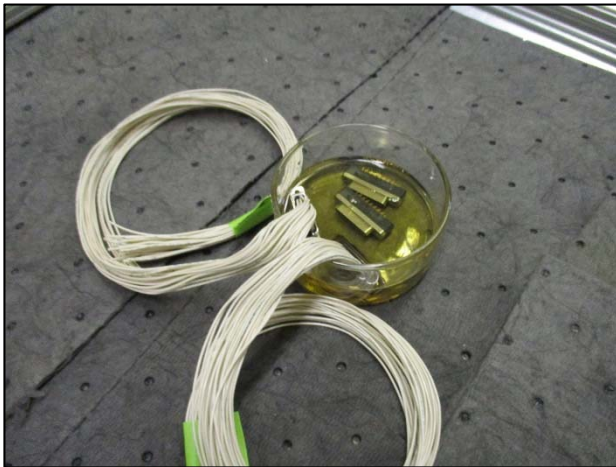
Figure 17 – Fluid Immersion Lubricating oil
