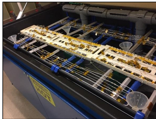
Figure 7 – Salt Spray Test Setup
