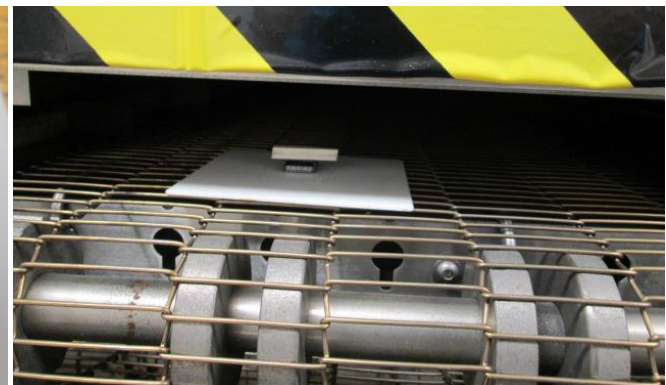
Figure 11 – Solderability Test Setup – Test Specimen on Oven Conveyor
