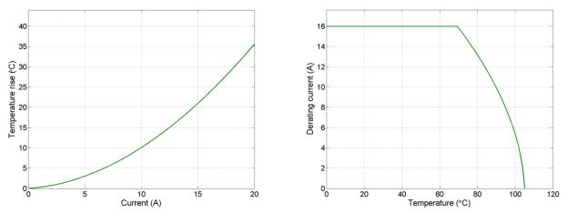
PS: The break-point of derating curve corresponds to the current 16.0A&69.6  $^\circ C.$
