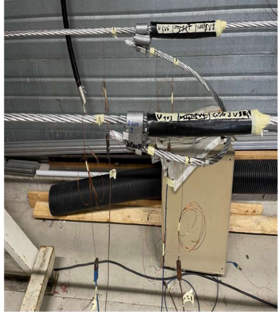
Fig 1: Representative photograph of Bolted Ampact Tap Connector P/N 2445483-1 test setup short-time current.
