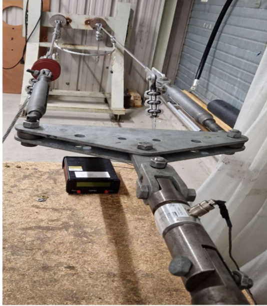
Fig 1: Representative photograph of Bolted Ampact Tap Connector P/N 2445483-1 test setup short-time current.
