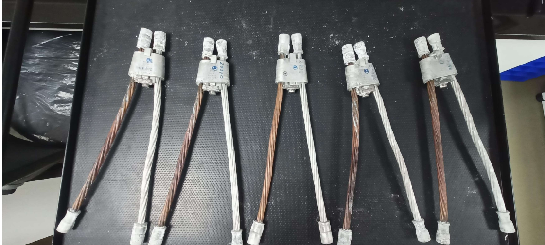
Fig 3: Samples after the salt spray test
