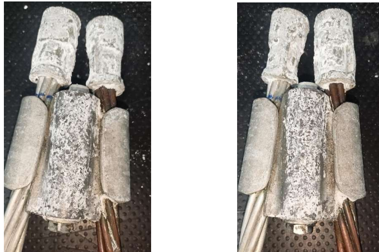
Fig 4: Samples after the salt spray test
