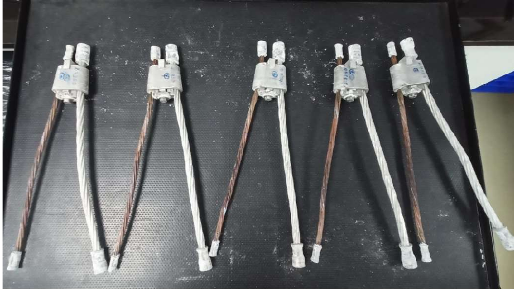
Fig 5: Samples after the salt spray test
