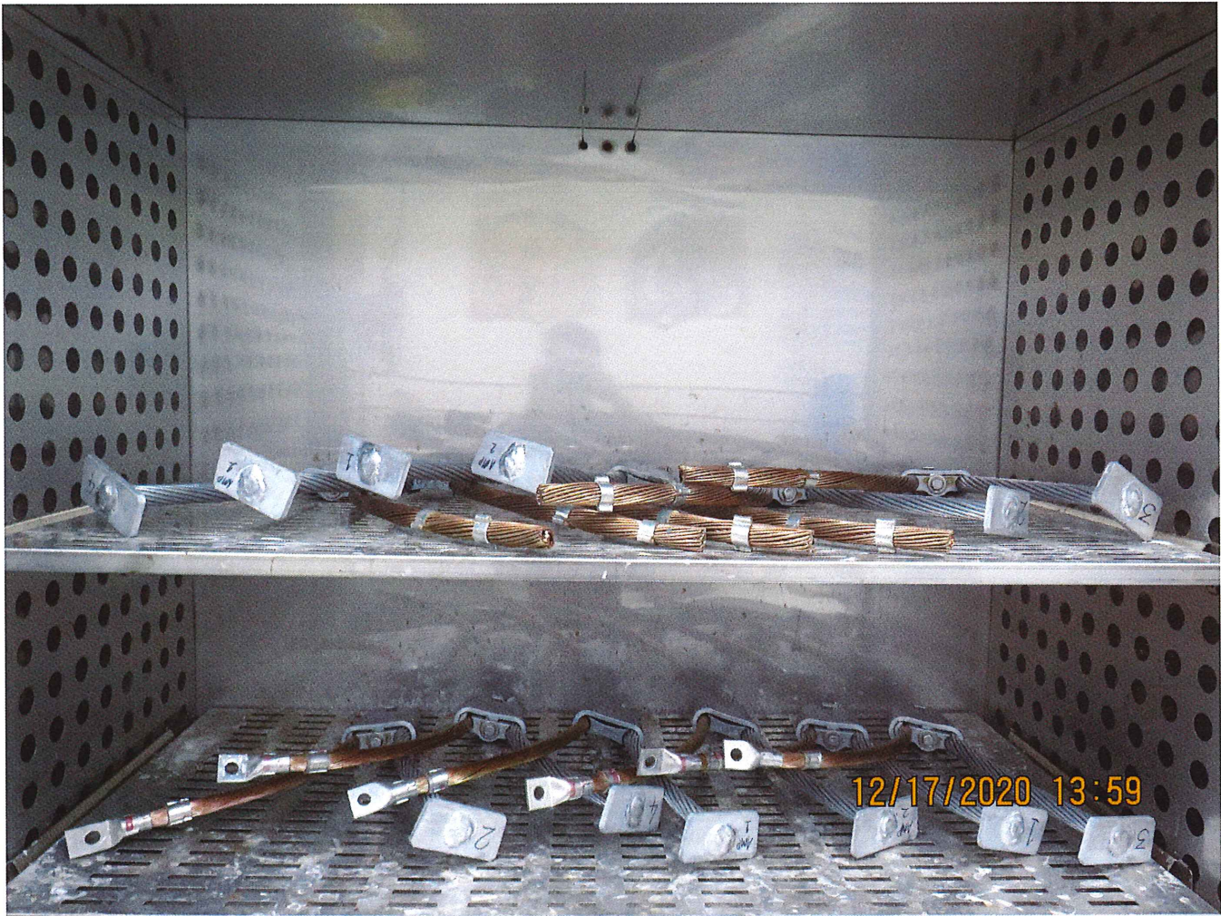
Photograph of AMPACT BAT Connectors set-up with all specimens for Thermal Shock Test to AMP Specification 109-13009
