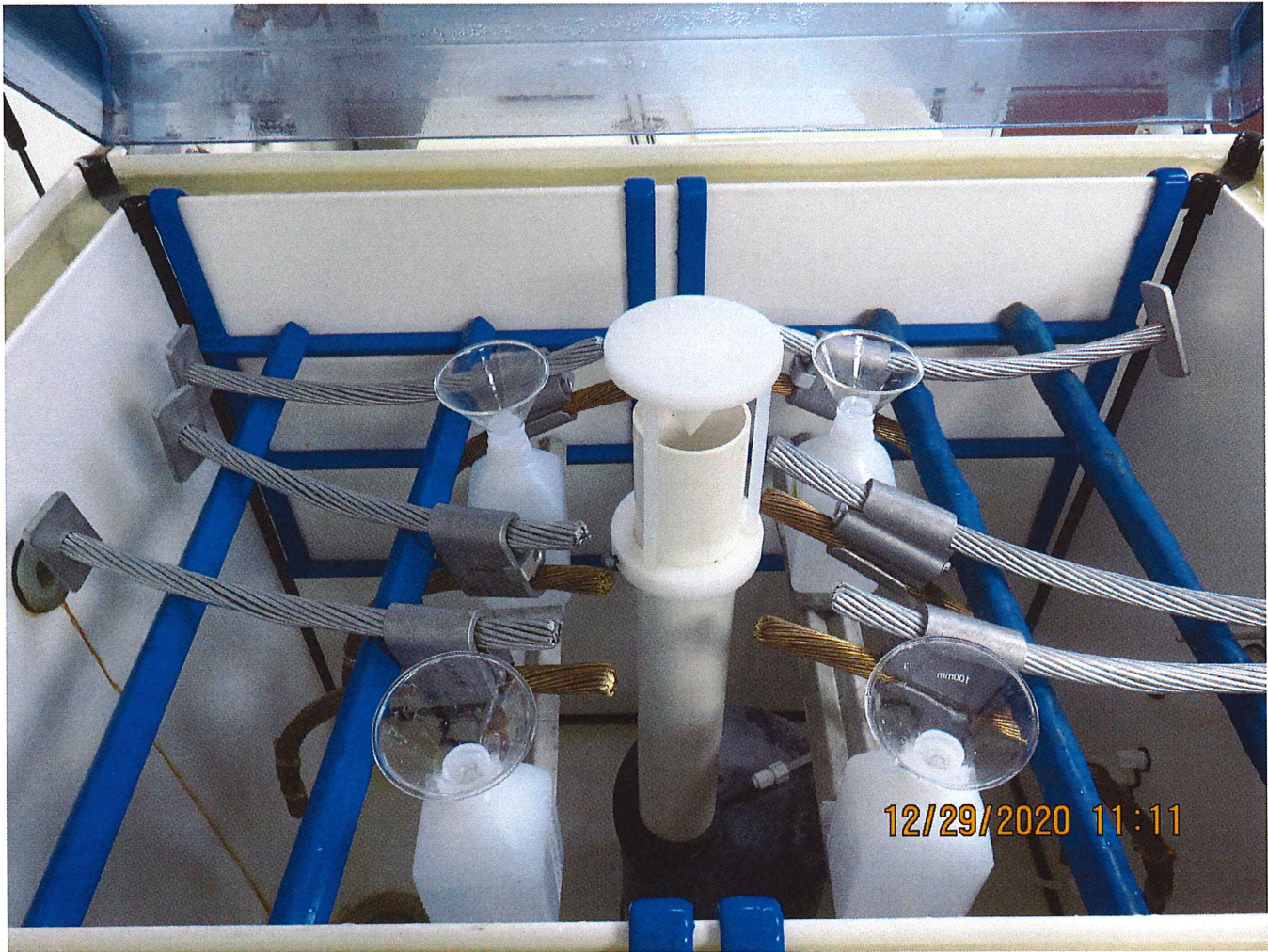
Representative photograph of AMPACT BAT Connector set-up during Salt Spray Test to EIA 364 – 26C
