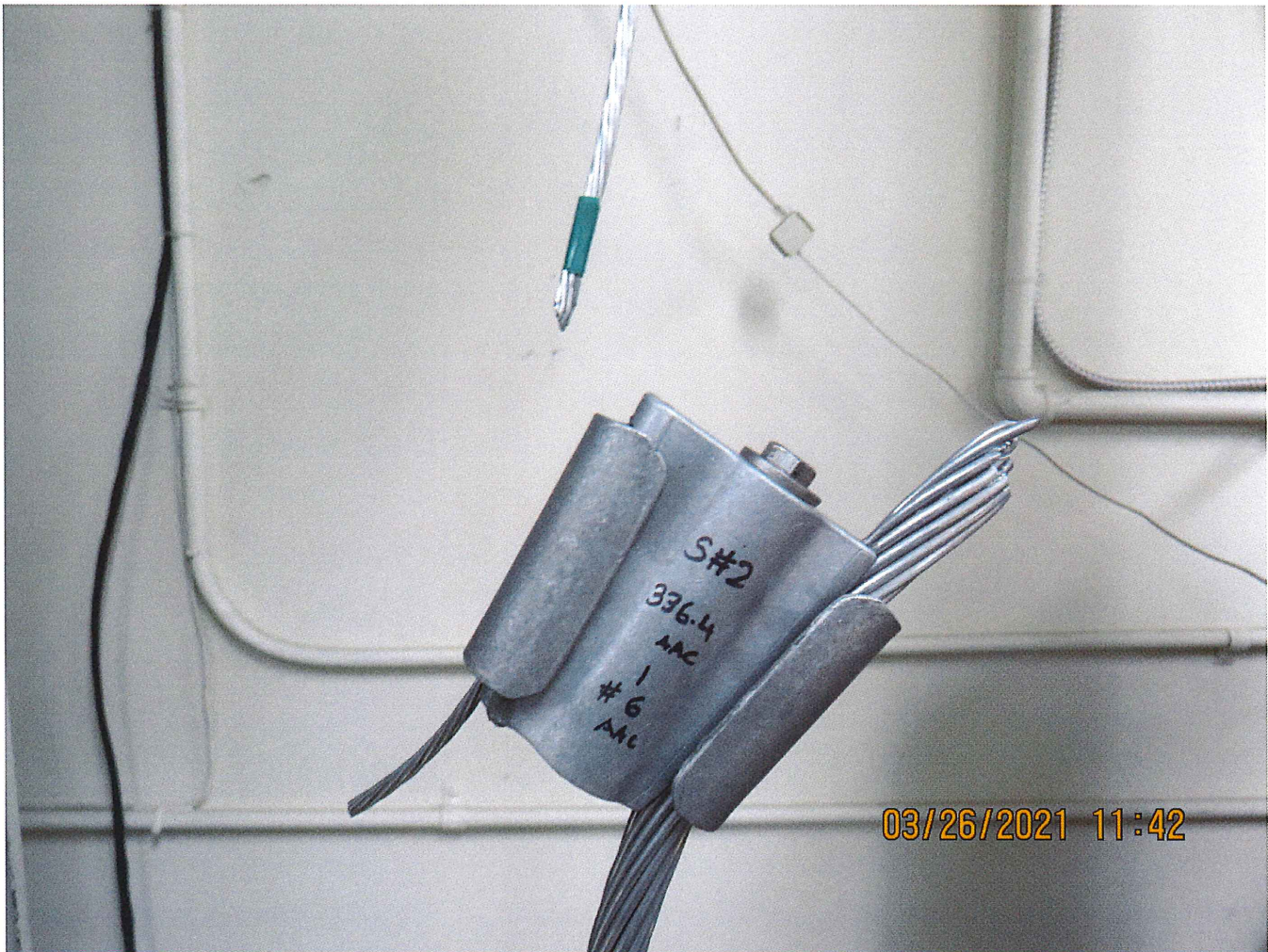
Representative photograph of AMPACT BAT Connector P/N 1-2376750-2 with 336.4 AAC and #6 AAC conductors after Mechanical Pull-Out, Class 3 Test to ANSI C119.4:2016
