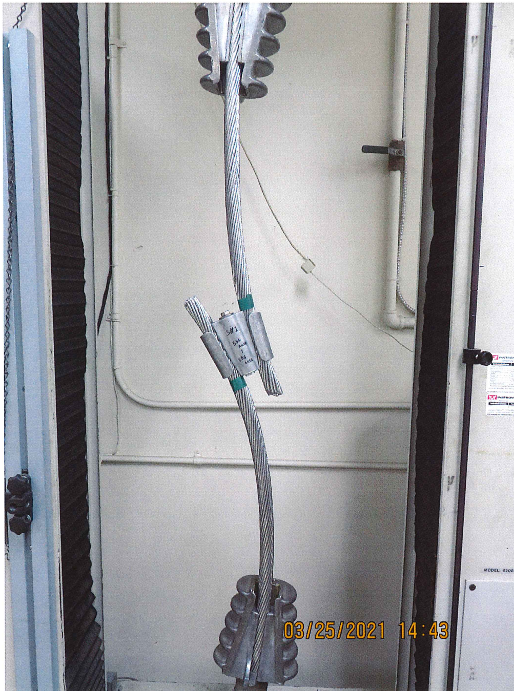
Representative set-up photograph of AMPACT BAT Connector P/N 2376750-1 with 556.5 ACSR conductors set-up for Mechanical Pull-Out, Class 3 Test to ANSI C119.4:2016
