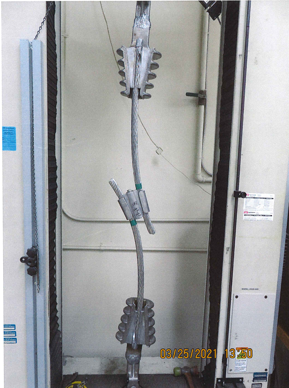
Representative set-up photograph of AMPACT BAT Connector P/N 2376750-1 with 556.5 AAC conductors set-up for Mechanical Pull-Out, Class 3 Test to ANSI C119.4:2016
