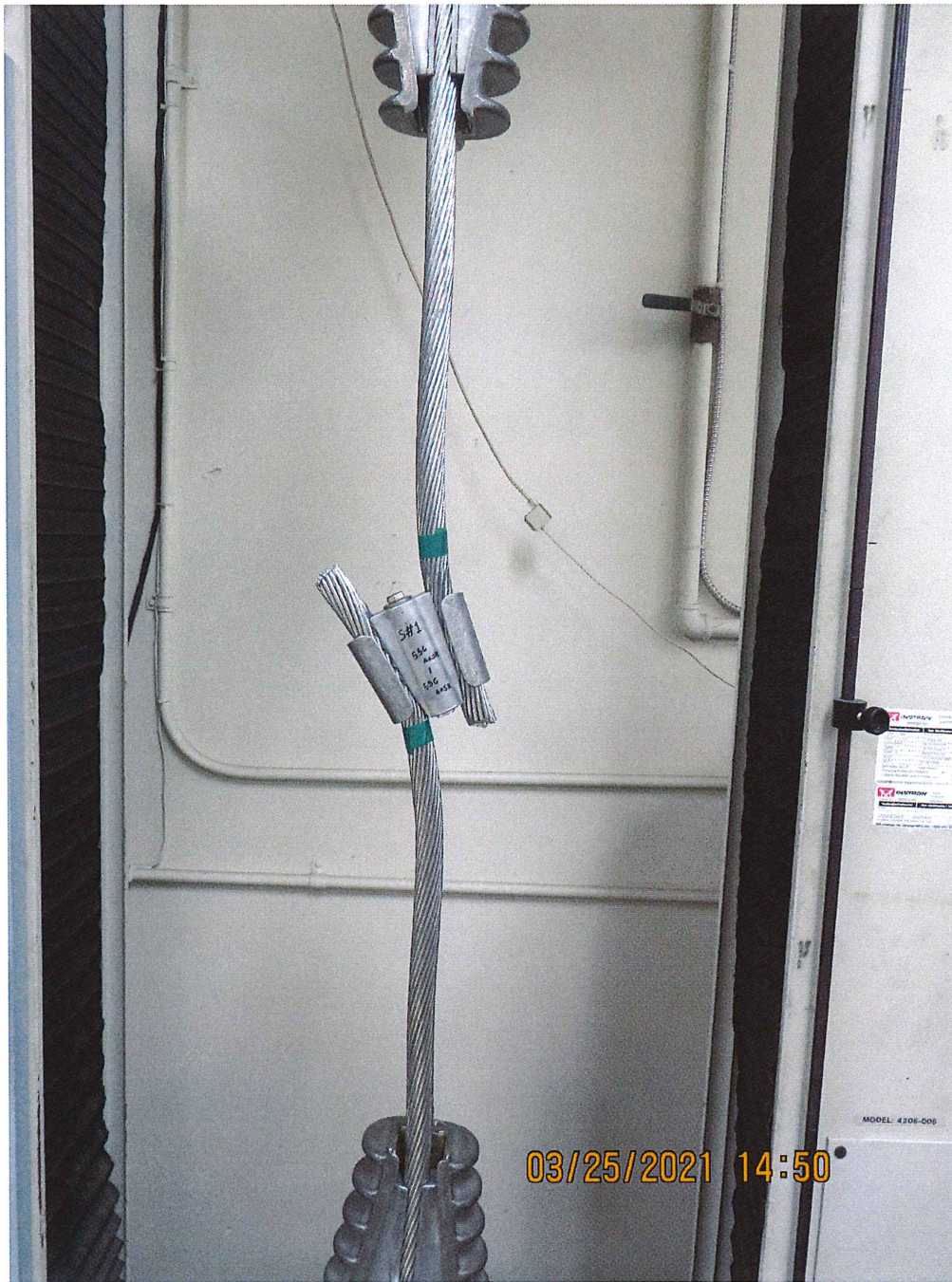
Representative photograph of AMPACT BAT Connector P/N 2376750-1 with 556.5 ACSR conductors after Mechanical Pull-Out, Class 3 Test to ANSI C119.4:2016
