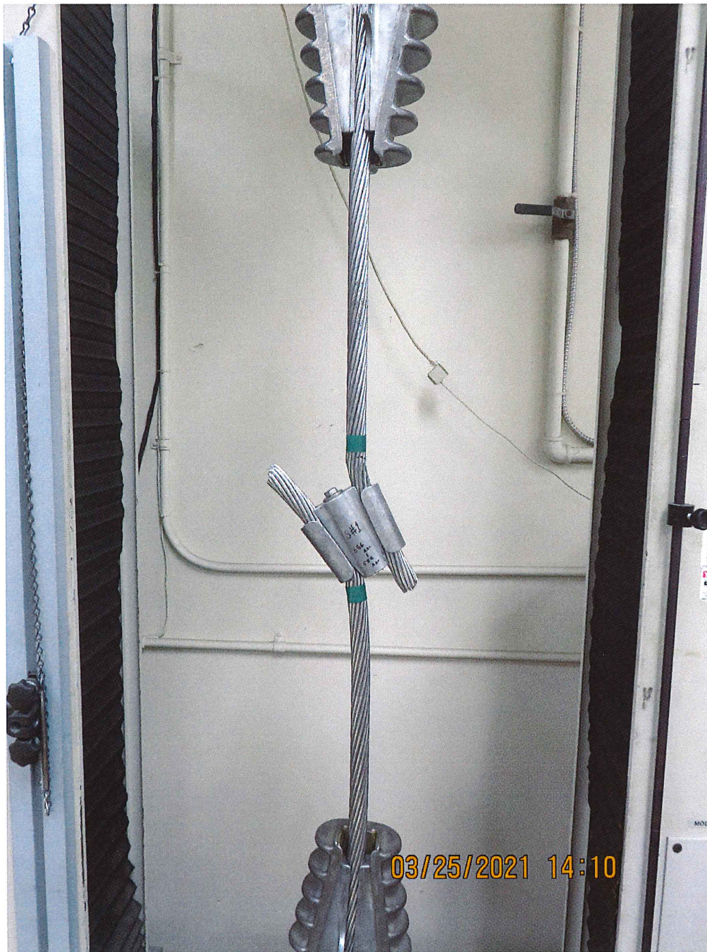
Representative photograph of AMPACT BAT Connector P/N 2376750-1 with 556.5 AAC conductors after Mechanical Pull-Out, Class 3 Test to ANSI C119.4:2016
