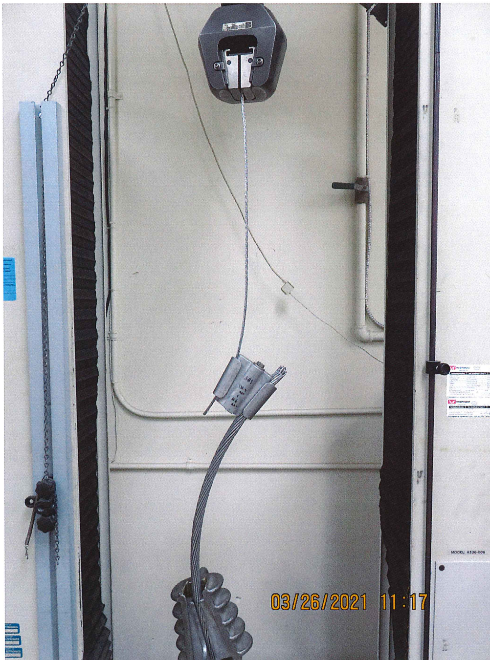
Representative set-up photograph of AMPACT BAT Connector P/N 1-2376750-2 with 336.4 AAC and #6 AAC conductors set-up for Mechanical Pull-Out, Class 3 Test to ANSI C119.4:2016
