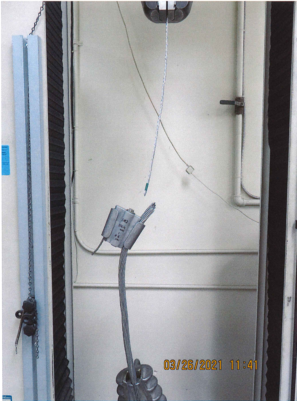
Representative photograph of AMPACT BAT Connector P/N 1-2376750-2 with 336.4 AAC and #6 AAC conductors after Mechanical Pull-Out, Class 3 Test to ANSI C119.4:2016
