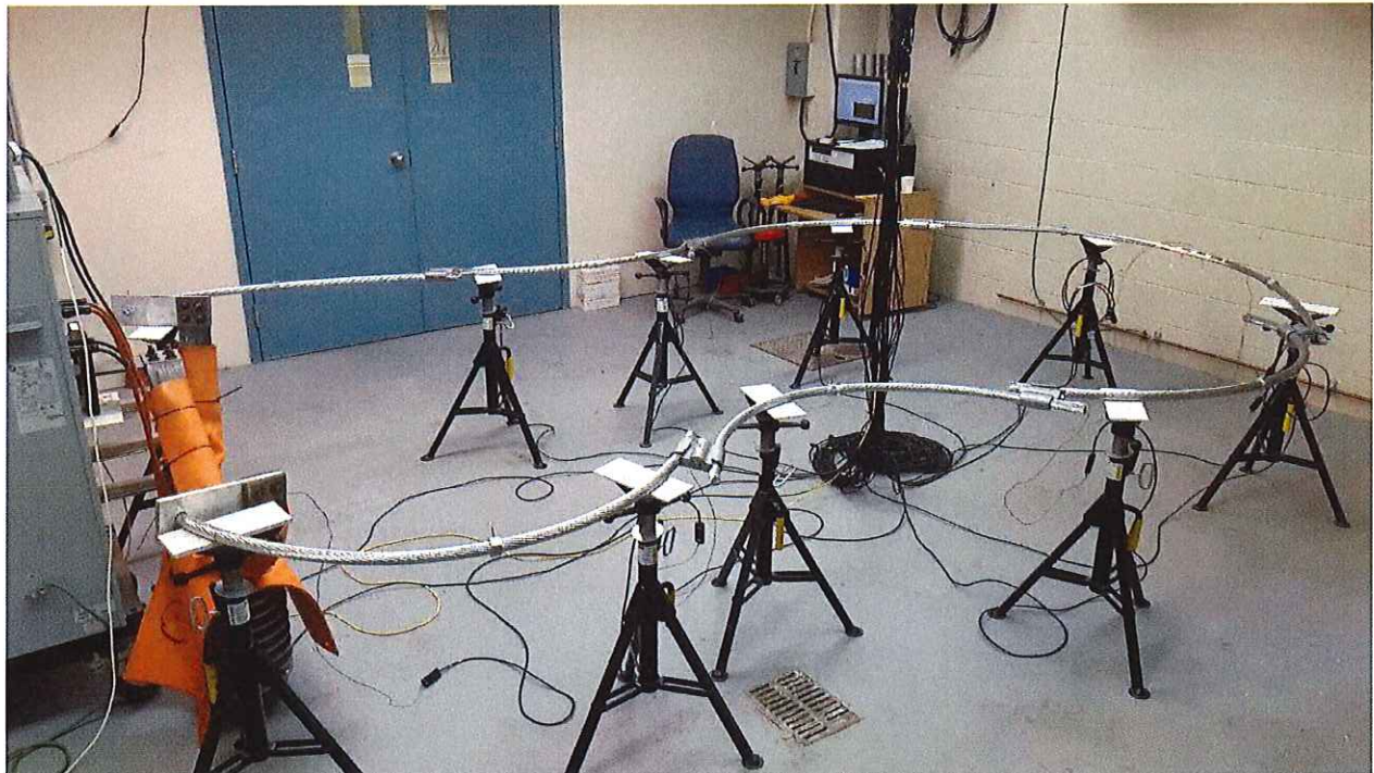
Photograph of AMPACT BAT Connectors set-up, 795AAC – 795 ACSR, with all specimens during Current Cycling Test to ANSI C119.4-2016 Class AA (Group 1)
