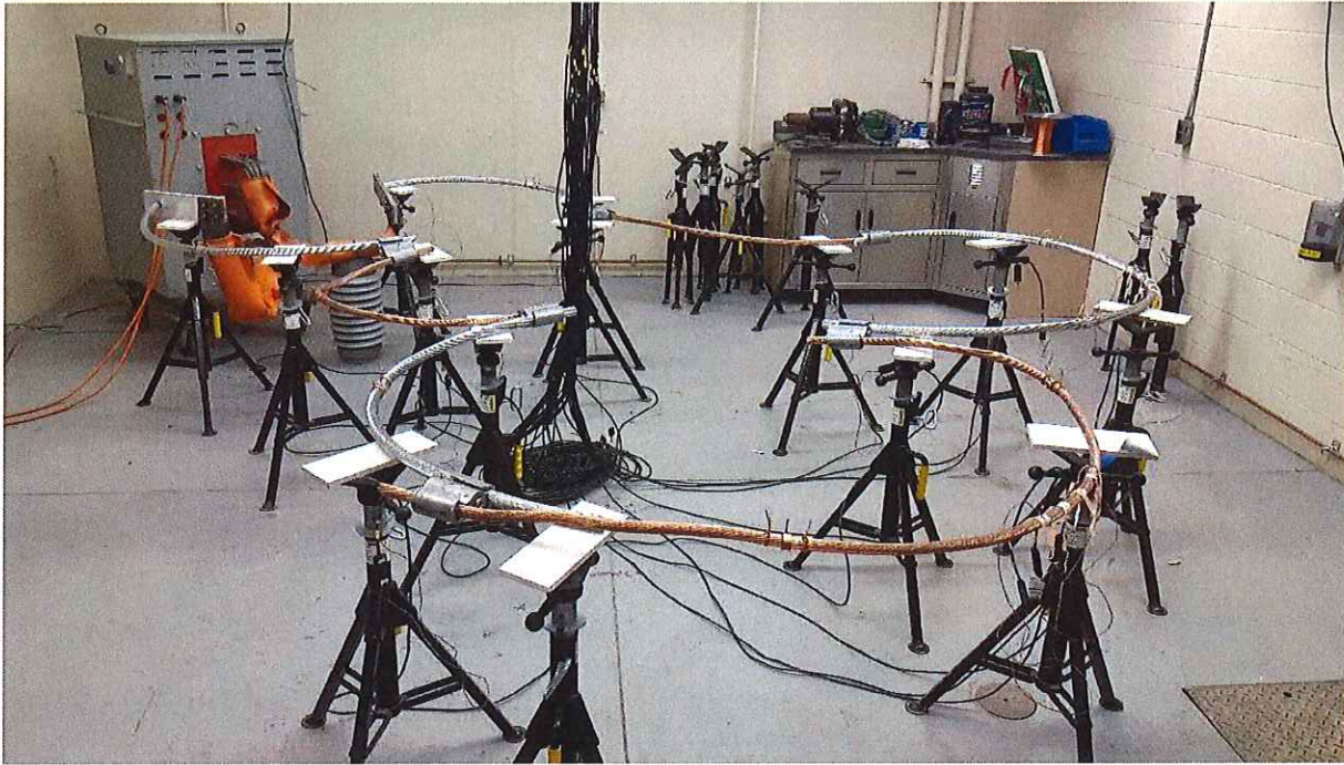
Photograph of AMPACT BAT Connectors set-up, 795AAC – 500 Cu, with all specimens during Current Cycling Test to ANSI C119.4-2016 Class AA (Group 2)
