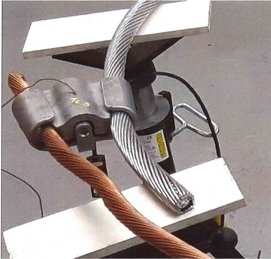
Representative close-up photograph of AMPACT BAT Connector, 795 AAC – 500 Cu, Current Cycling Test to ANSI C119.4-2016 Class AA (Group 2)
