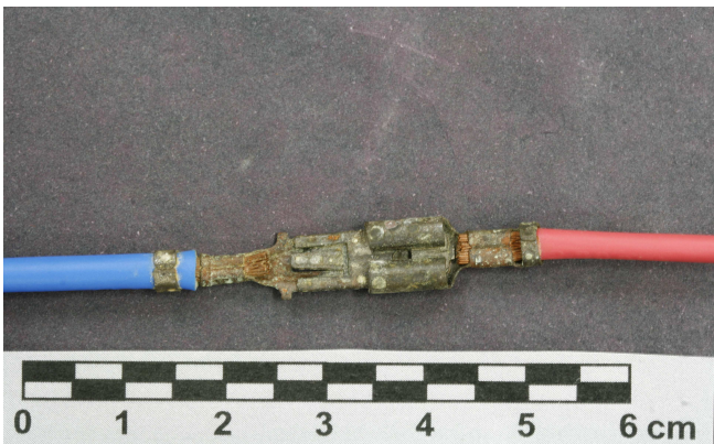
Figure 4: Samples without housing (original test) after sulfur dioxide exposure test FORMBR-0697 Mar/2007
