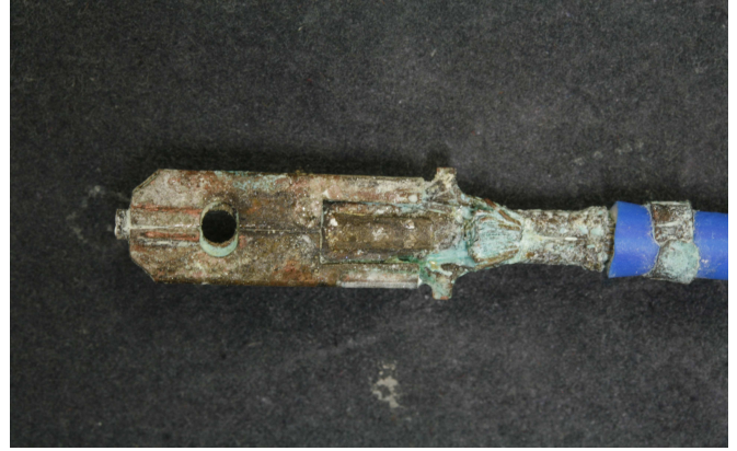
Figure 7: .250 Fastin-on Tab (housing removed) after sulfur dioxide exposure test
