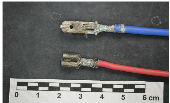
Figure 5: Samples with housing (removed to take the picture) after sulfur dioxide exposure test RL130432 Pag. 7 de 10
