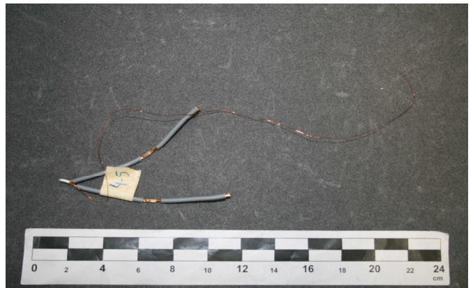
Picture 4: Combination IV - 2 X 18 AWG Copper Wire + 1 X Ø 0,20mm Aluminum Magnetic wire
