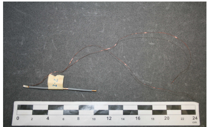
Picture 2: Combination II - 1 X 18 AWG Copper Wire + 1 X Ø 0,20mm + 1 X Ø 0,16mm Aluminum Magnetic wire
