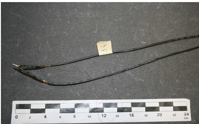
Picture 3: Combination III - 2 X 20 AWG Copper Wire + 1 X Ø 0,16mm Aluminum Magnetic wire
