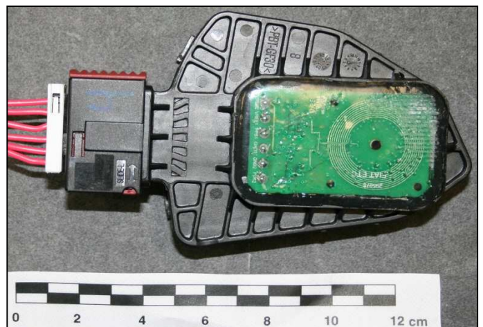
Photo 6 - HSG 6 POS. assembled to FIAT counterpart
