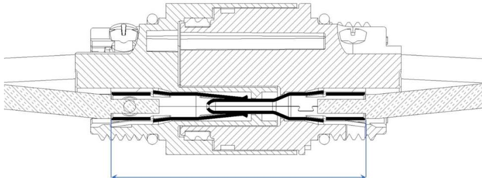
**Figure 1, In-Line connector**
