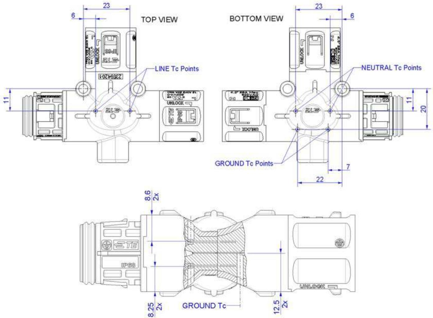
Figure 5, Drawing for drilling holes
