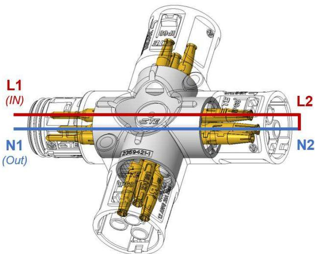
Figure 4, Straight Circuit
