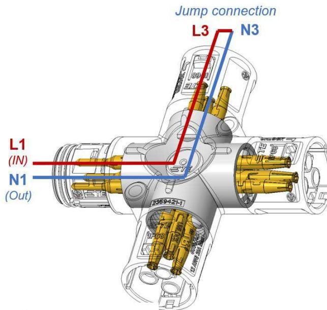
Figure 3, Branch Circuit
