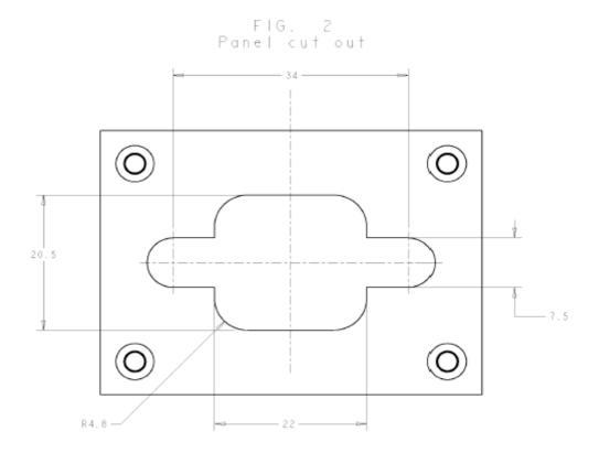
Steel plate, Ni plated, thickness 1,9mm 0 +0,1 Missing dimensions per drawing 1577134
