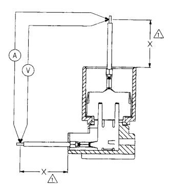
VOLTAGE DROP DUE TO X INCHES OF WIRE IS TO BE REMOVED FROM ALL READINGS.
