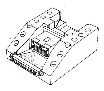
Figure 3 Mounting and Clamping Locations for Vibration and Physical Shock
