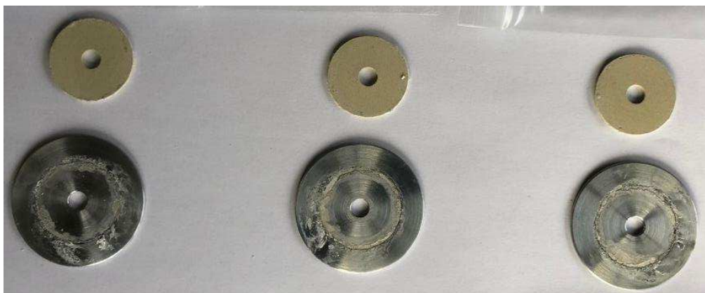
Aluminium 6061-T6 coupons and their associated Silicone Silver Aluminium gaskets after 504 hours of salt-fog exposure.
