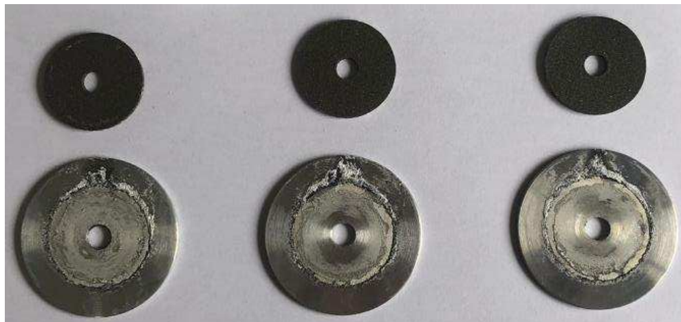
Aluminium 6061-T6 coupons and their associated Silicone Nickel Graphite gaskets after 504 hours of salt-fog exposure.
