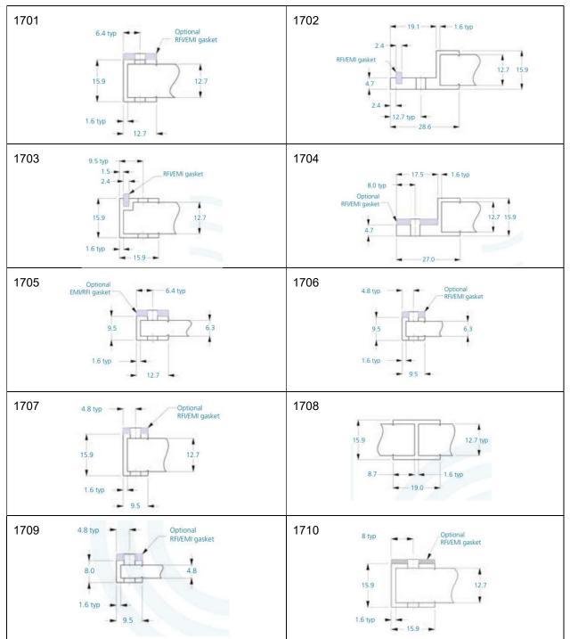
Note: 1702 and 1704 the 'front face' is classified as the face without the gasket at the bottom of the section view.
