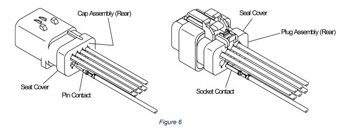
3. When all the required contacts have been inserted, complete the assembly by pushing the TPA into the fully locked position. The plug housing TPA may be fully locked by holding the rear of the housing assembly and pushing the TPA toward the rear of the housing.
