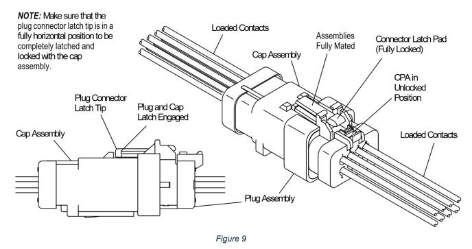
7. By pushing the CPA toward the plug housing, it can be slid into the locked position in which it slides under the connector latch pad. See Figure 10.
