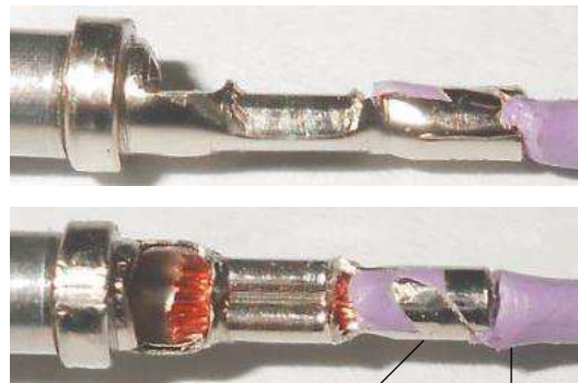
Skewing of Wire Insulation Acceptable Slight Deformation of Wire Insulation Acceptable
