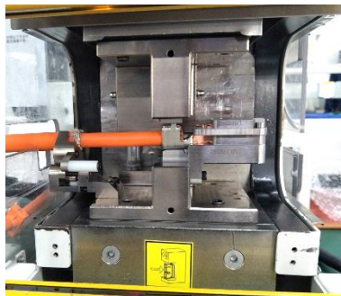
Figure1: PCON21 contact 180deg crimping applicator
