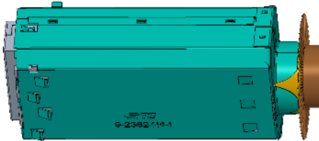
Figure 10: Raising screening braid
