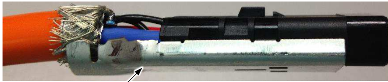
Shield on Bottom of Inner Housing (Shown)
