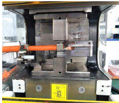
Figure1: PCON21 contact 90deg crimping applicator
