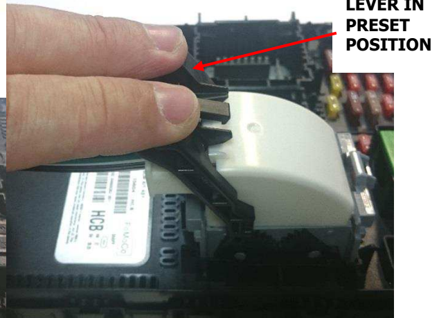
Figure 26: Unmate connector by moving lever back into the pre-lock position
