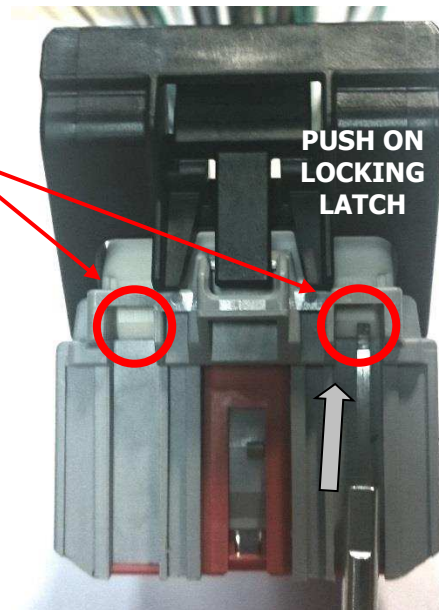
Figure 16: Unlock of wire dress cover
