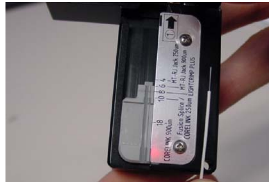
11. Remove the fiber, which is now cleaved to the proper length.
