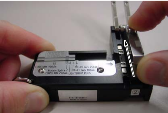
3. Press down on the button and slide the carriage back (in the direction shown).
