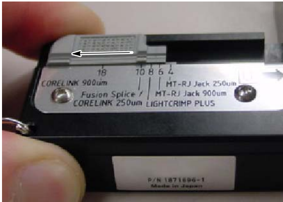
4. Move the fiber slide back until it stops.
