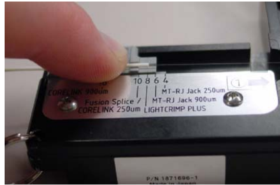
6. Place the stripped and cleaned fiber into the slot at the desired cleave length.
