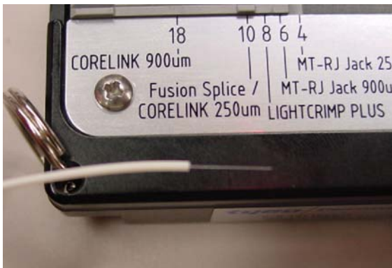
12. Remove the fiber, which is now cleaved to the proper length.
