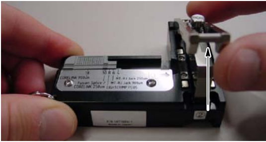
2. Open the fiber clamp.
