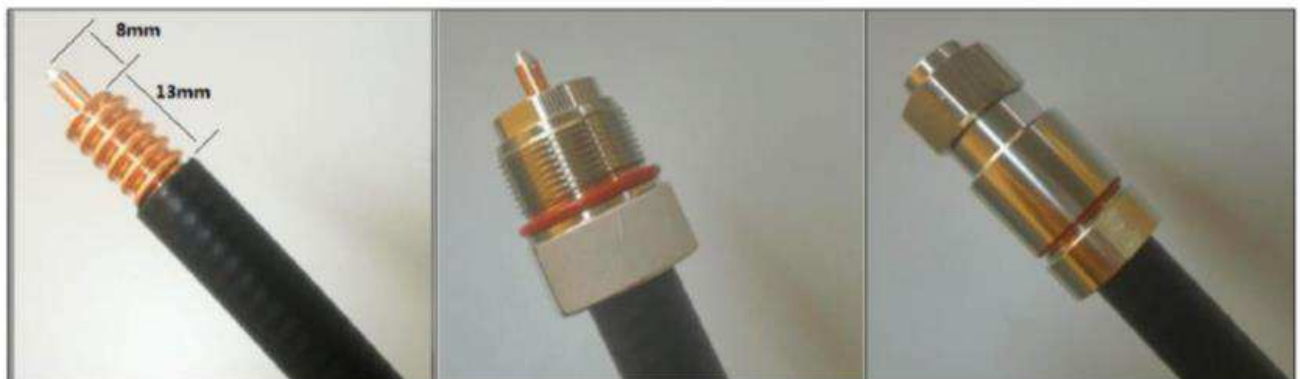
4. 截取合适的长度，去除毛刺，内导体倒角 4. Get the request dimension, chamfering and deburr at inner conduct, brush the chipping
