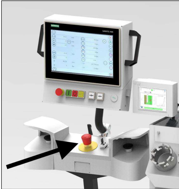
Figure 19: Emergency stop button.
