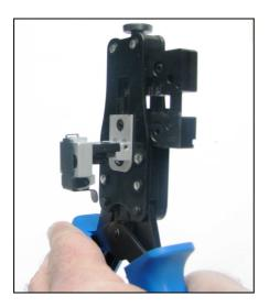
Picture 3: Swinging out the contact locator
