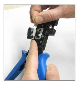
Picture 5: Inserting the contact up to stop into the contact locator
