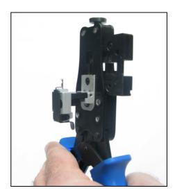
Picture 6: Retaining the contact in position
