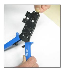
Picture 4: Moving and retaining the crimping die set
