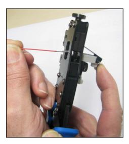
Picture 9: Removing contact from crimping die set
