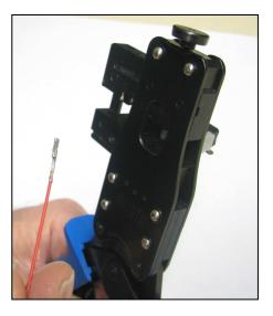
Picture 10: Checking the crimped contact
