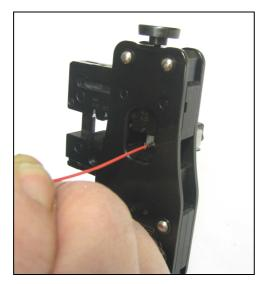
Picture 7: Inserting stripped wire in to the crimp sleeve of contact up to wire stop
