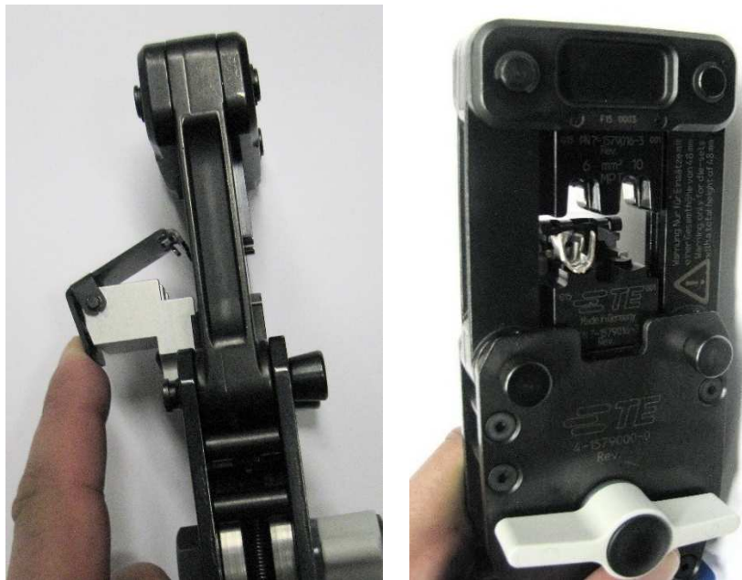
Abb. 3: Terminal holder opened (left), terminal positioned (right)
