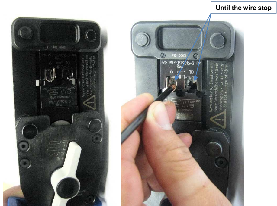
Abb. 4 : Terminal positioned (left), insert wire to wire stop (right)
