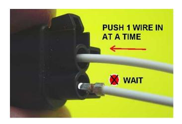
**D2** - After insertion of a contact, pull back the wire lightly in order to check if the contact is securely locked in position. Do not twist the wire or contact when lightly pulling!
