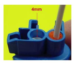
If removal of a cavity plug is necessary, it can be removed by pushing from the front of the connector with a thin point. Do not reuse the cavity plug if damaged.
