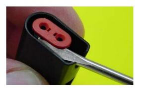
**G1.2:** The contacts can then be extracted by placing an extraction tool (or small screwdriver) between the contact and the tip of the primary locking arm and gently lifting it up to clear the contact:
